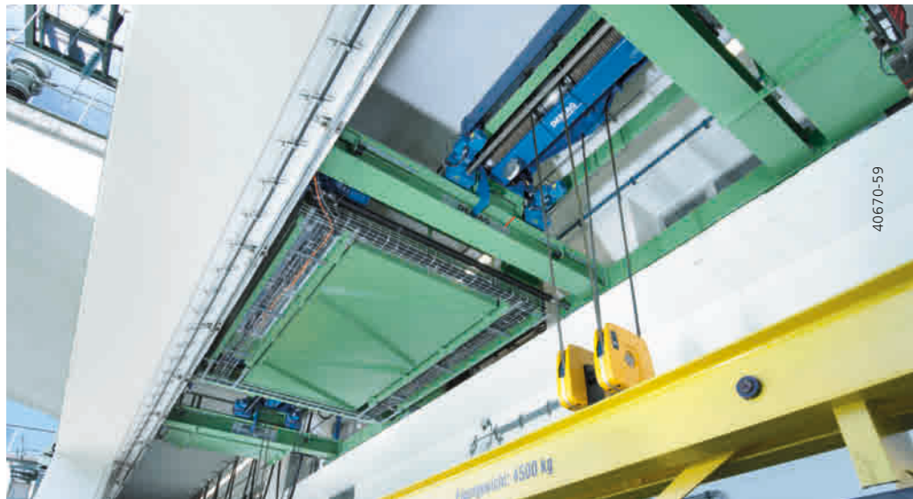
Dam beams are positioned with 2 DH hoist units at water depths of up to 22 m.
