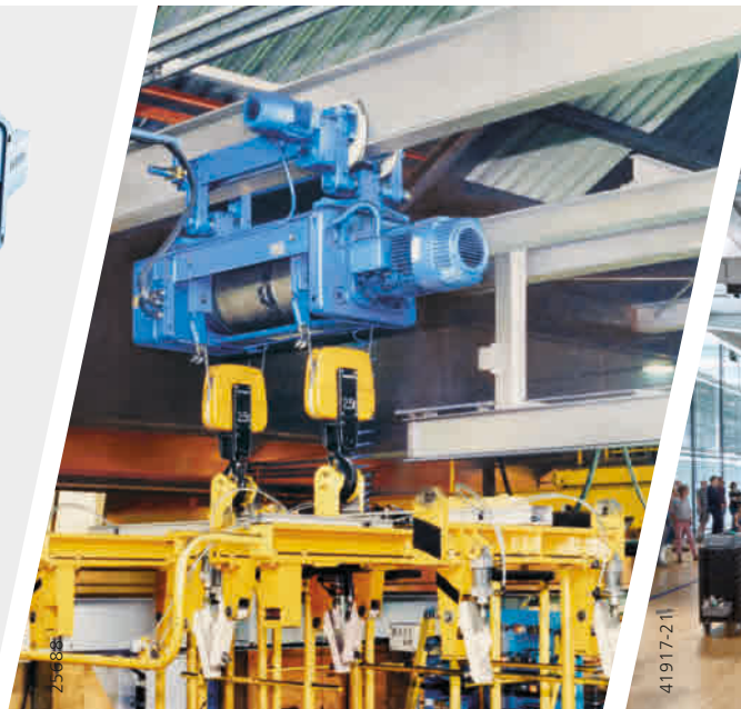
DH hoist unit with two rope lead-offs for transporting mould jigs without any hook travel
