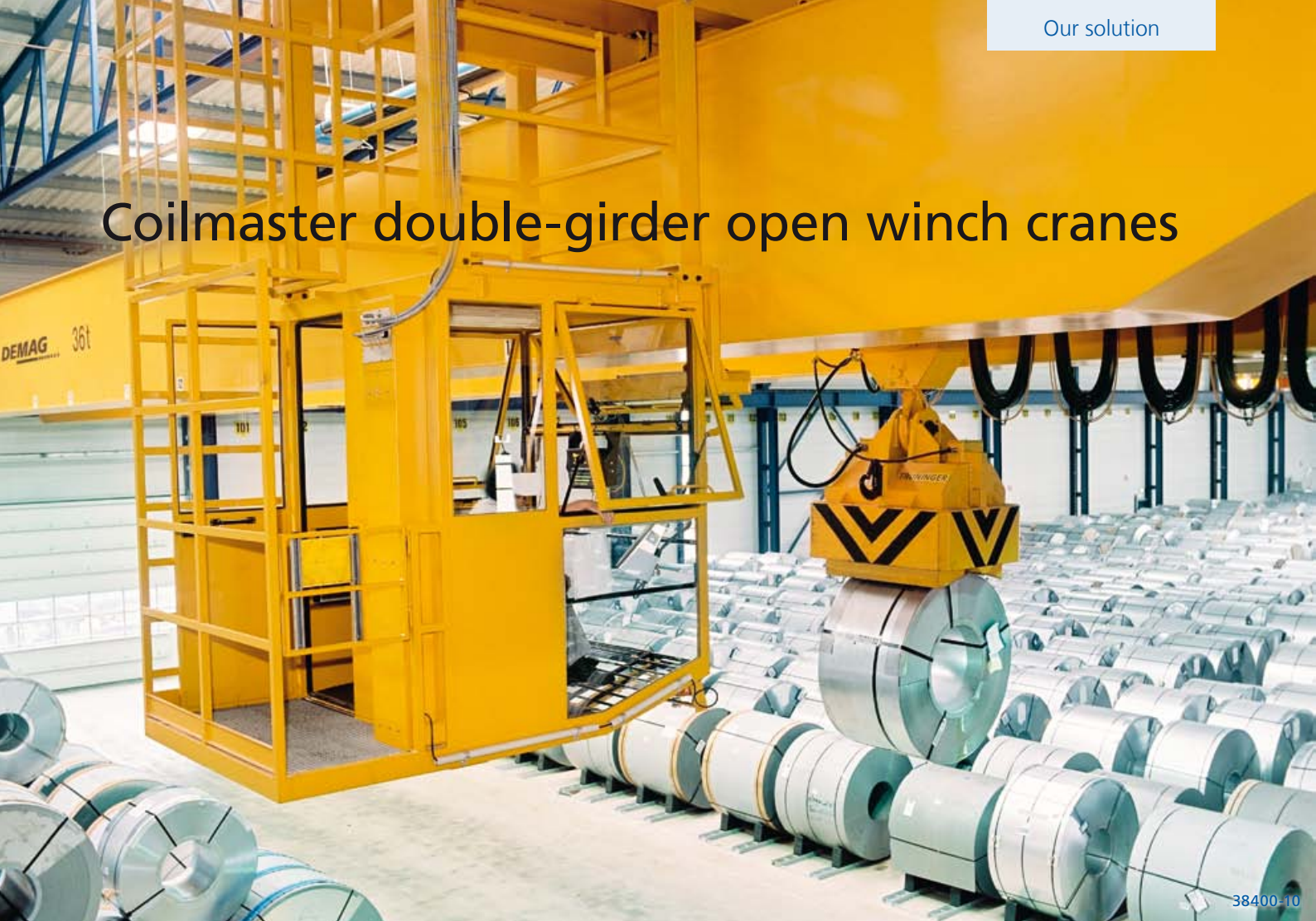
Coilmaster double-girder open winch crane with cab control
