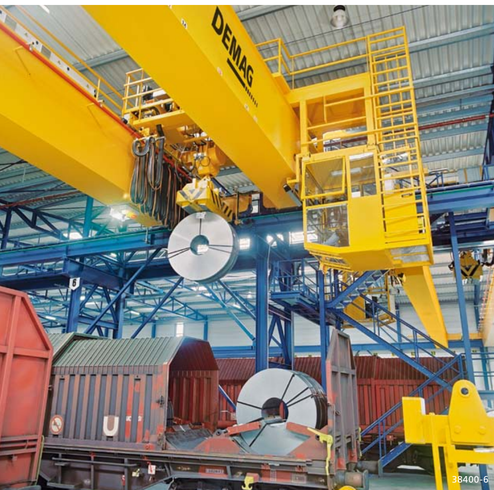
Coils being delivered by train in a steel service centre
