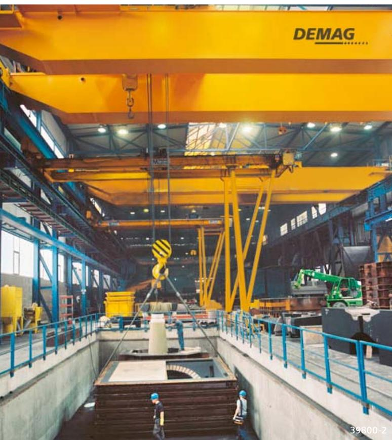
The casting ladle is precisely positioned and molten iron is safely and reliably transported to the casting machine in a foundry
