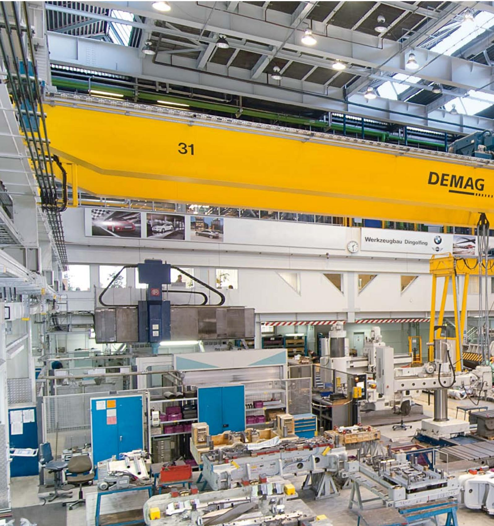
Double-girder semi-portal cranes for maintenance work on press tooling at an automotive production facility
