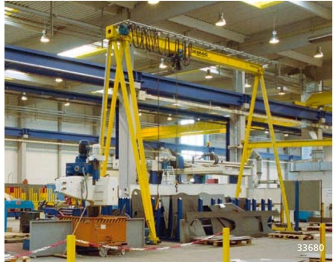
Demag's single-girder full-portal cranes are similar in construction to semi-portal cranes. The main difference is in the integrated pivot portal legs which compensate for crane motions. Full-portal cranes can often be integrated in existing production environments and in-plant logistics with little construction work.
