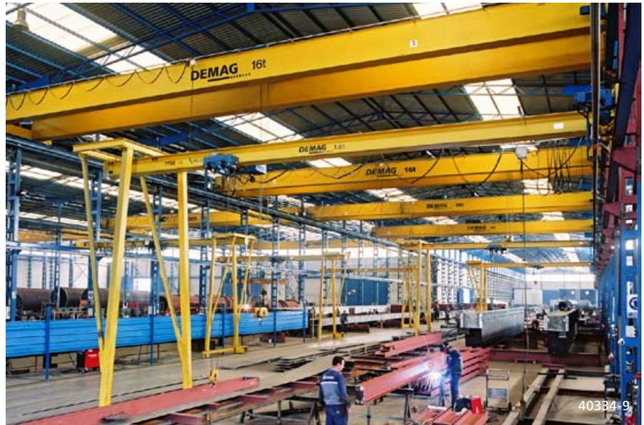
In addition, portal cranes can also be installed as workplace or loading cranes under bridge cranes. This fully integrated solution offers additional flexibility and increases productivity per square metre.
