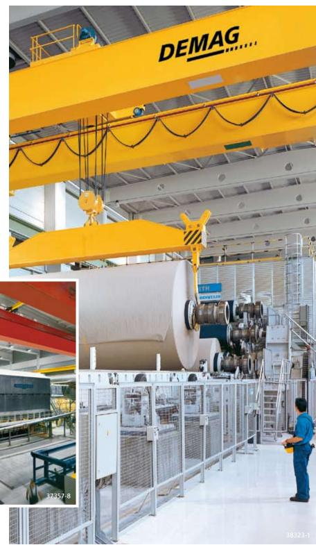
Changing rolls and cylinders: Demag double-girder crane for safely changing rolls at the wet end of the paper machine.
