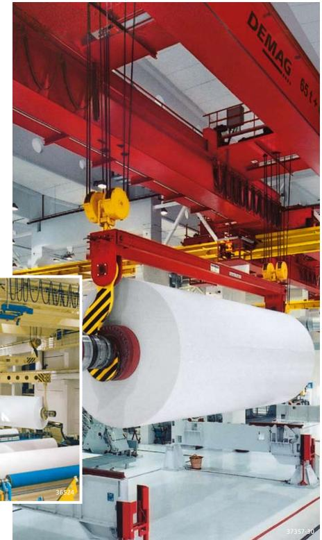
Paper finishing: Demag double-girder crane with motor-powered spreader bar for reel transport between intermediate storage and finishing.
