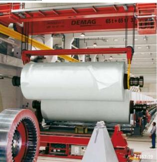
Reel transport: Intermediate storage of paper rolls before transport to the rewinder.
