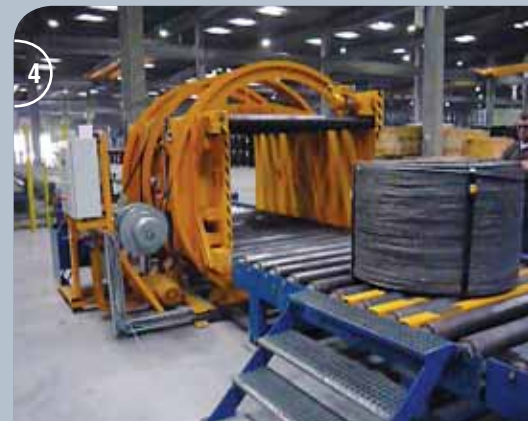
1-4 Elektromotorische Coilwendestation. Electromotive coil turning station.
