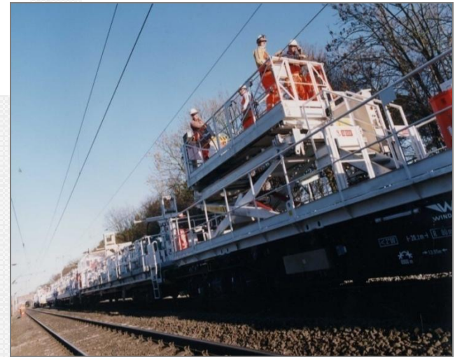
Re-Wiring Train in Multitraction, 8 Engines, 2120 kW
