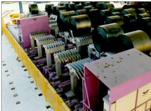
Interdepartmental coil transport from hot line 500°C. Customer: Voest-Alpine Stahl, A-Linz
