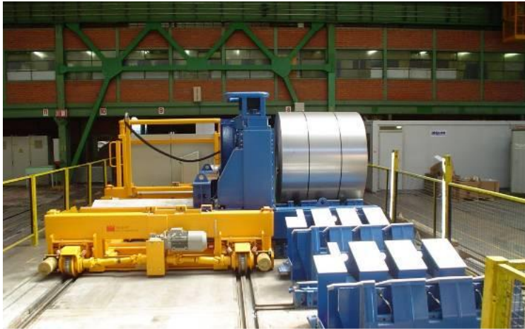
Coil transport vehicle, load capacity 30 to Customer: Ugine & ALZ
