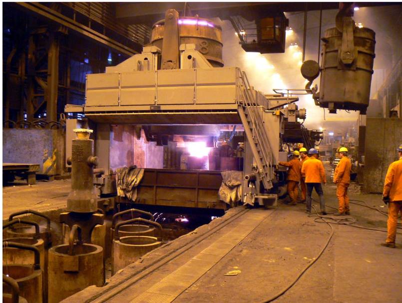
Casting Car 110 t with hydraulic lifting device and crosswise sliding equipment Customer:: Stahlwerk Bous
