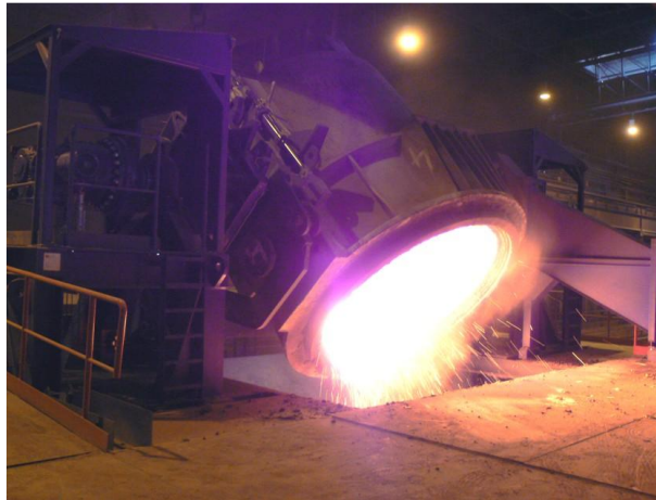
Ladle roll-over device. Load capacity:: 90 to Customer: Ugine & ALZ, Gent
