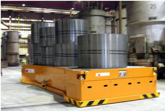
2 Coil transport vehicles, load capacity 180to each. Radio remote-controlled for use at batch annealing Client: Thyssen Krupp Stahl, Bochum
