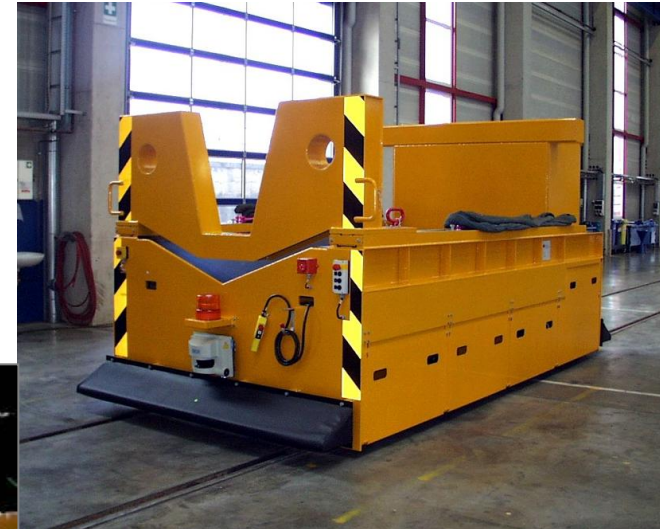
Coil transport vehicle, batterie-electric drive and a capacity load of 50 to. Client: Toscelik, Türkei
