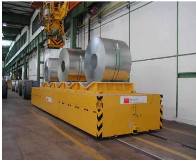
Coil transport vehicles, load capacity 96 tons Client: Salzgitter Flachstahl GmbH
