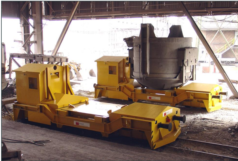
Scrap metal transport vehicle with 90to load capacity Custmer: Elwood Steel Belgium
