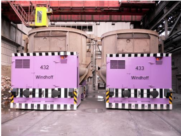
Scrap hopper transport car 155to, Customer: DEW Witten
