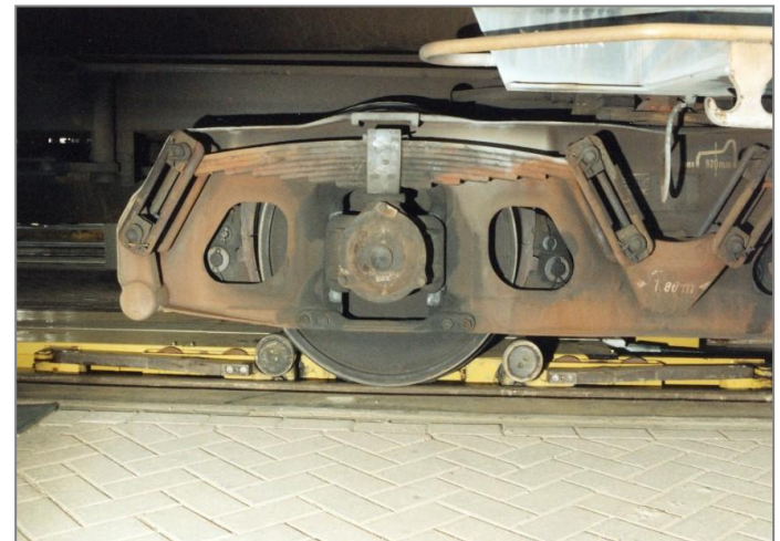
Wheelset cart: Pressure roller pair engaged.
