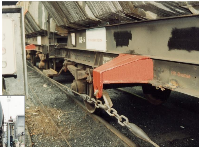
Reversible rope winch, here with sling chain and C-hook for pulling forces up to 30 kN (for UIC application).
