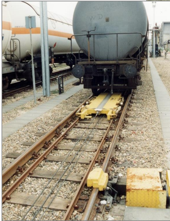
Wheelset cart in combination with an automatic drag shoe placing for track safety.
