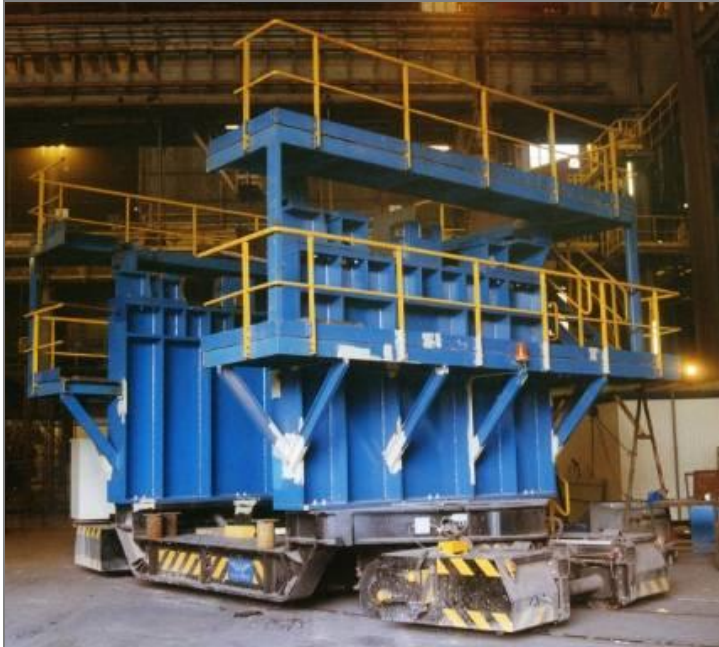
Segment transfer car with bogies, Load capacity: 140 tons, Customer: Sidmar, Gent
