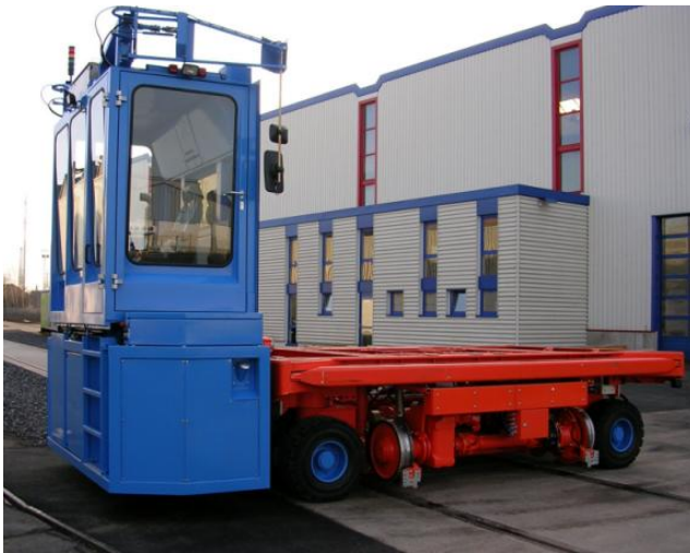
Road/Rail Pallet Transporter for liquid aluminium laddles- and anodes up to 40to
