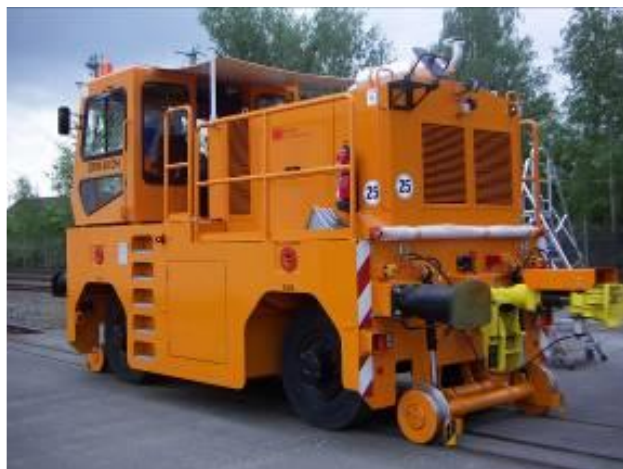
ZRW 60 DH, Tractive force: 1200 to Batterie-electric drive Customer: BASF Ludwigshafen
