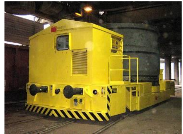
Scrap metal transport vehicle with 90to load capacity Customer: Swiss Steel, Switzerland
