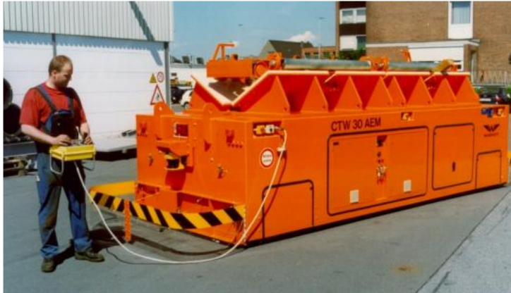
Magnetic line guided coil transport vehicle CTW 30 AEM. Customer: Krupp Thyssen Nirosta, D-Krefeld
