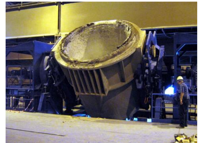
Ladle tilting device Load capacityt: 230 to Customer: Ugine & ALZ, Gent
