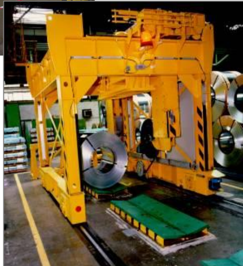
Coil transport vehicles with 4 tilting devices and a load capacity of each 35 tons Client: Sidmar
