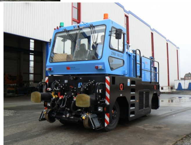
ZRW 140DH with diesel-hydraulic drive, Tractive force: 2.800to Customer: Neuss Düsseldorfer Häfen
