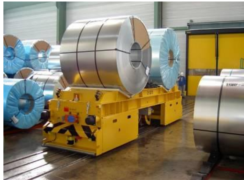
Coil transport vehicle, load capacity 2 x 32 to. Clientr: Thyssen Krupp Stahl, Ferndorf
