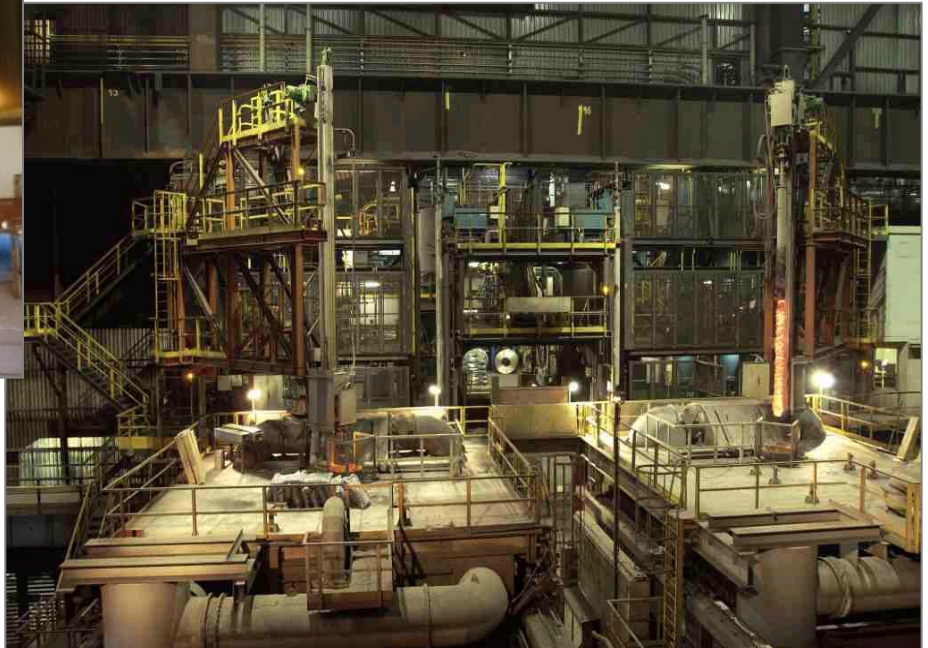
2 Hooded handling carts for flue gas extraction for pig iron desulphurisation Customer: Voest Alpine, Linz, Austria
