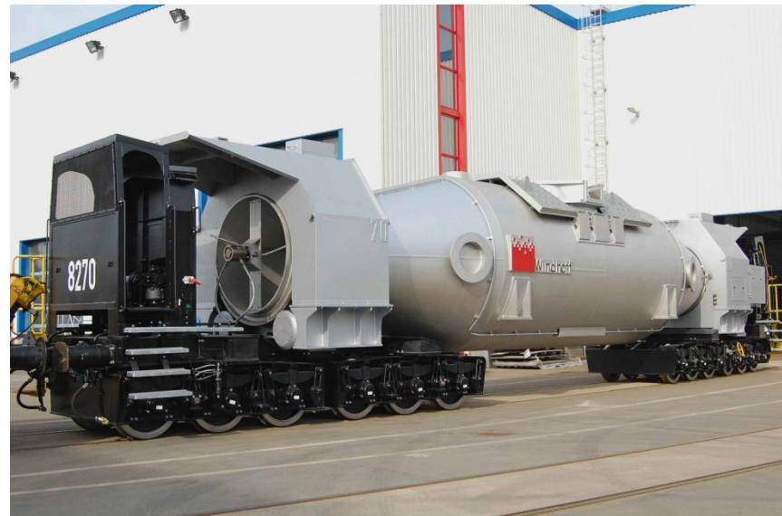
Torpedo ladle vehicle, ladle payload 200 tons Vehicle service weight: 190 tons ; Gross weight: 390 tons
