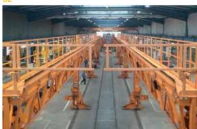
01: Integrated roof access plattform, vertically and longitudinally adjustable (universal service stand)
