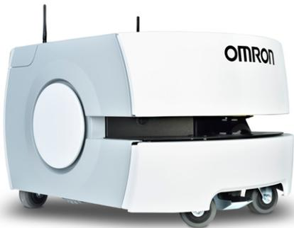
Omron LD mobile robot is also available in cleanroom rating: Fed Class 100, ISO Class 5
